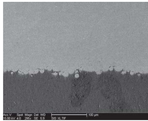
Fig. 5 Secondary electron image of the interface between the cold sprayed coating and the aluminum substrate
